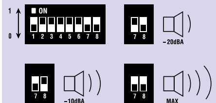
Sound selection 1 to 5, output level 7 & 8, 6 not used
